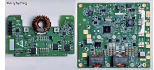
Photo by Tigo Energy Left: Tigo Energy Maximizer integrated junction box; Right: modular DC buck-boost box from SolarEdge. The circuit boards are meant to give readers a chance to compare electronic component count of a Tigo Energy Junction Box and a SolarEdge PowerBox
